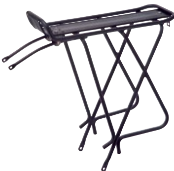
City / Commuter YA-16E Alloy DIECAST (ADC10) frame and steel wire stays With clip, foldable Adjustable brackets Fits: 24", 26", 27", 28" Max. load: 18 kgs
