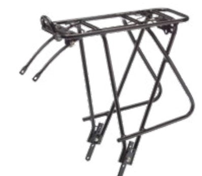
City / Commuter / Touring YA-91J Alloy tube frame and stays With clip Adjustable stays and brackets Max. load: 25 kgs
