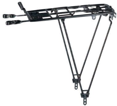
City / Commuter YA-7B Alloy DIECAST (ADC10) frame and steel wire stays With clip, foldable Adjustable brackets Fits: 24", 26", 27", 28" Max. load: 18 kgs
