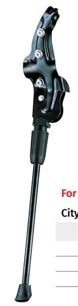
SPECIALLY DESIGNED ANGLE The bracket can be retracted under the chainstays when it is kicked up and will not protrude, preventing your heels from being accidentally hit. E-bikes / City / Commuter / MTB YRA-81 ADC10 with plastic feet Big angle, fit bikes with disc brakes Adjustable: 24" - 29" Max. weight: 18 kg
