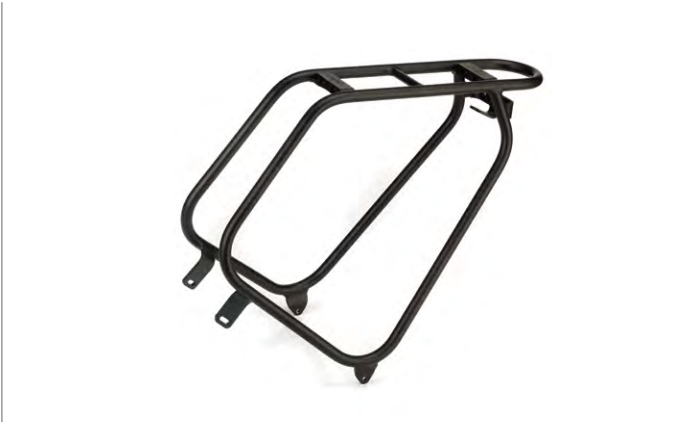
CUSTOMIZED CARRIER: For reference / information purpose only Full suspension e-bikes YA-255A Aluminum carrier Snap-it, AVS quick-release system available 4-POINTS FIXED Max. load: 20 Kg
