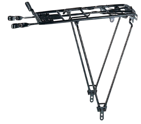
City / Commuter YA-7B Alloy diecast (ADC10) frame and steel wire stays With clip, foldable Adjustable brackets Fits: 24", 26", 27", 28" Max. load: 18 kg
